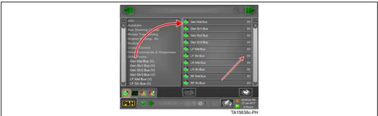
Figure 23. Bus voltage indication
